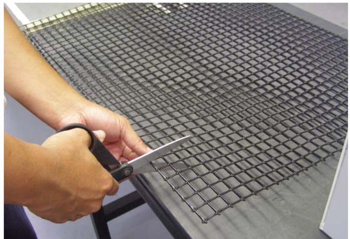
REME filter media custom cut to required size
